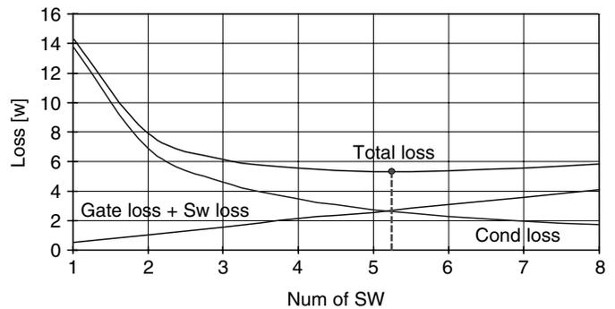
**FIGURE 1.11** Switching Loss, Gate Drive Loss, and Conduction Loss of an IRL3803 Versus a Parallel Switch Number
