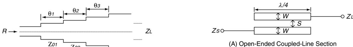
FIGURE 7.11 Multi-Section Impedance Transformer
